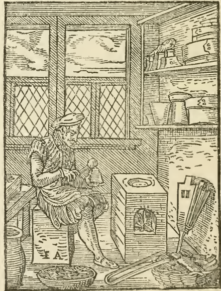
Type-Casting as Practised in 1564. [From Jost Amman.]
